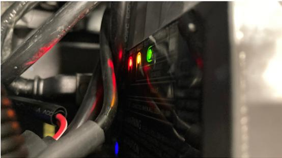
Start by turning the key off, with vehicle in neutral. Connect the charger cord to your charging port and verify the LED on the cord is on, as well as the LED on the charging port. Next, check that the three LED's are lit on the end of the charger itself. These lights should indicate at least a boot-up sequence, indicating there is boot-up power available.
